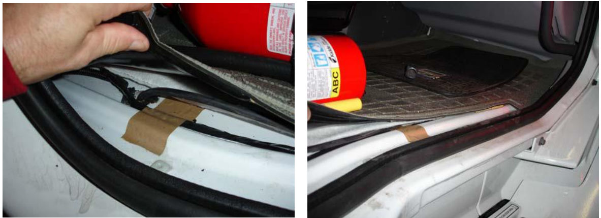
Figure 29 Sample Cable Placement in a Vehicle Cab
